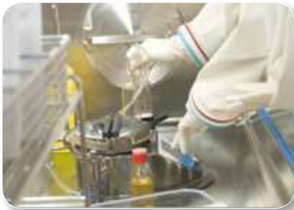
Esco Turbulent Flow Aseptic (Grade A) Isolator provide a safe and clean environment for aseptic production.
